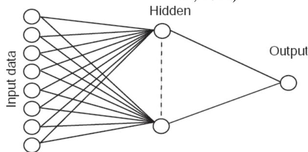
Fig. 2: Schematic diagram of MLP (Gil and Johnsson, 2010)
